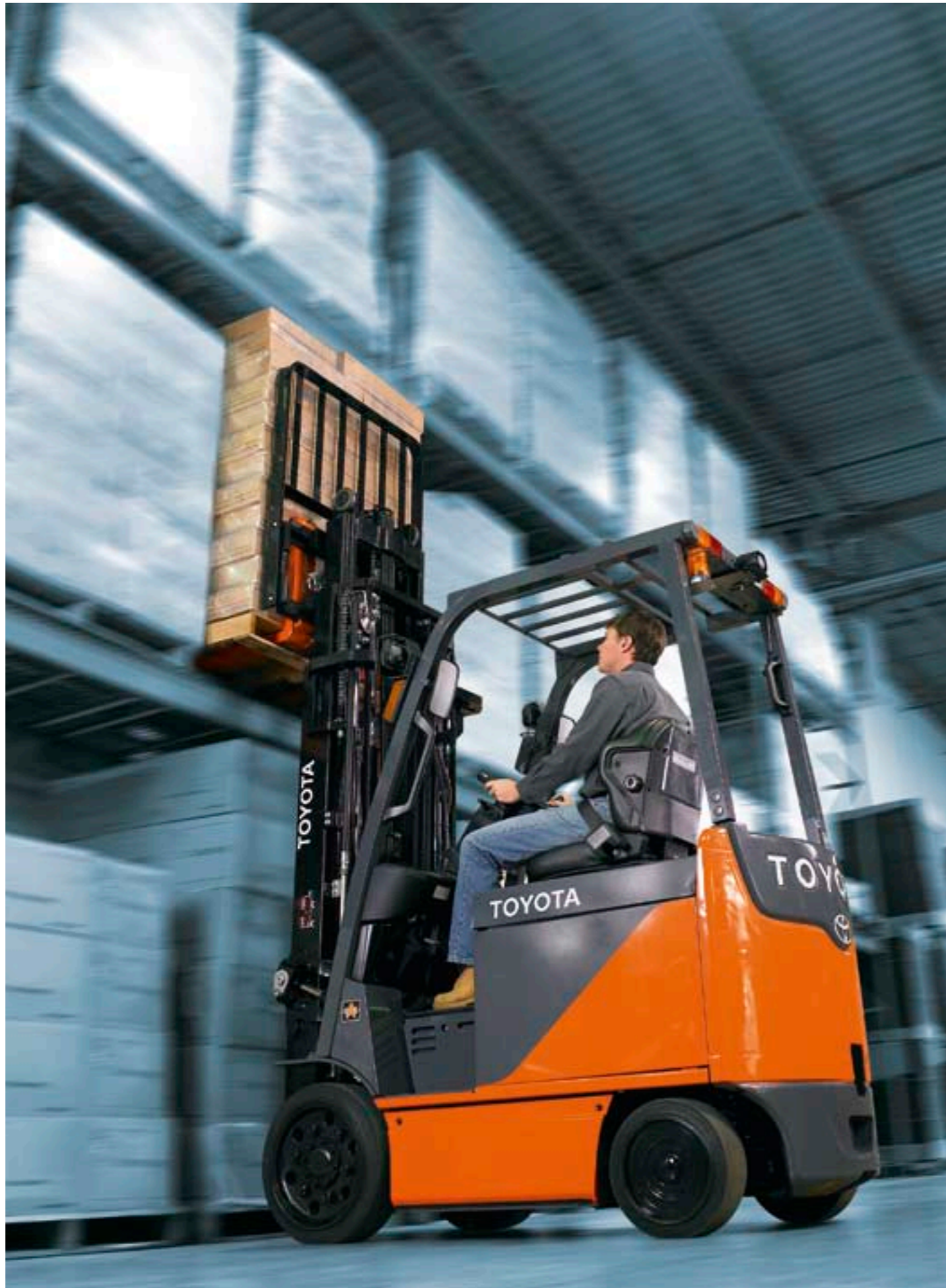
Access all areas. Cushion tyre trucks are significantly narrower than their pneumatic tyre counterparts.
