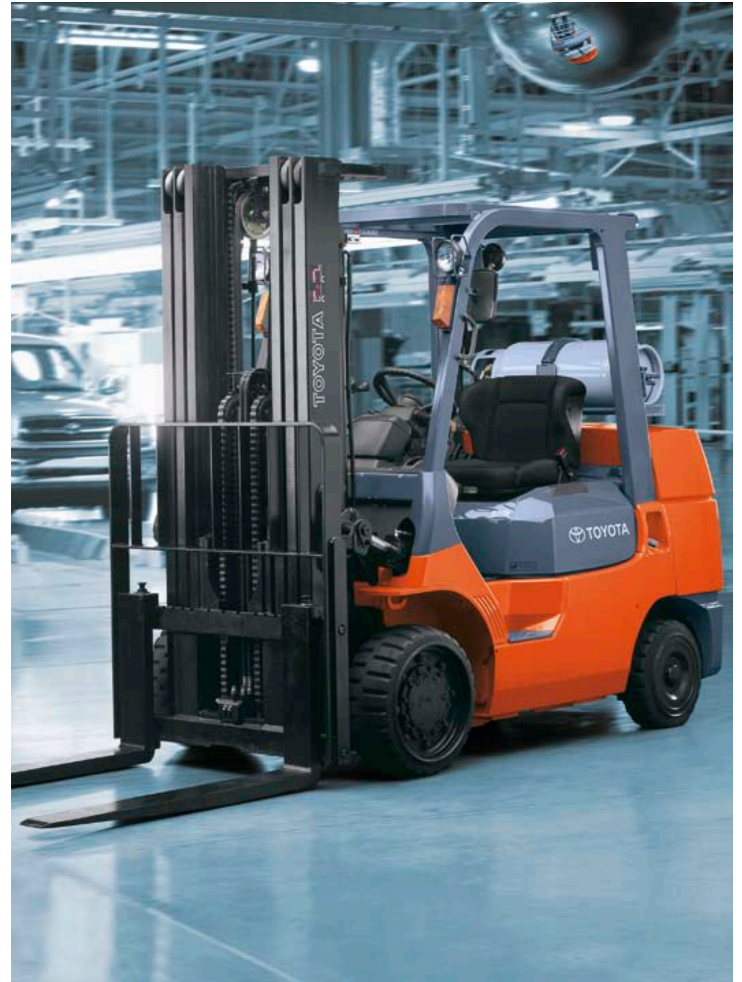
Perfect for narrow alleys: Cushion tyre trucks operate efficiently in narrow alleys thanks to their compact dimensions.
