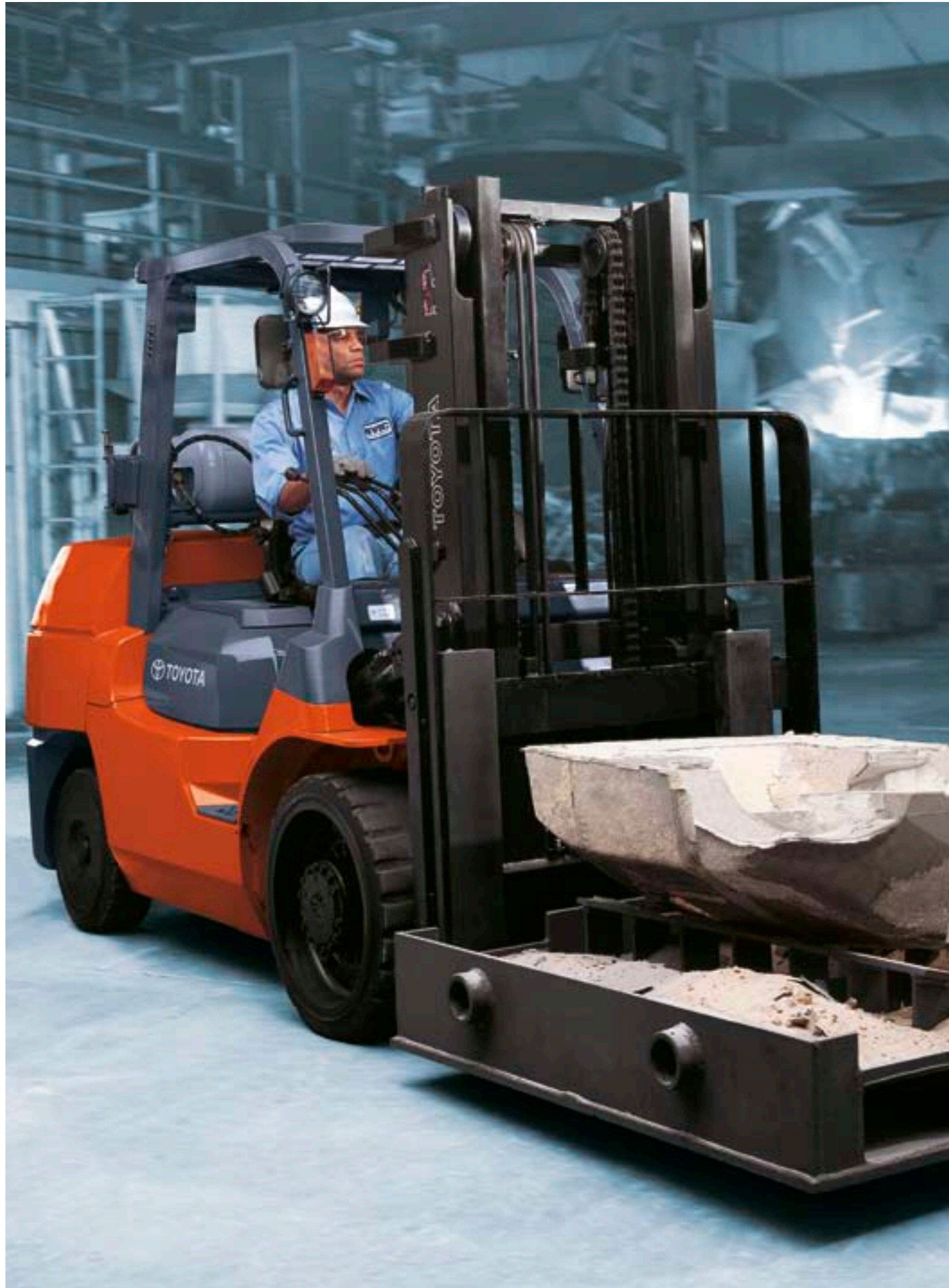
Heavy load handling: Cushion tyre trucks with LPG engines can lift loads up to 7.0 tons; the electric-powered versions can handle loads up to 3.0 tons.
